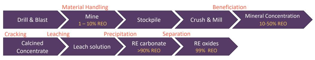
Hard rock mining, complex metallurgical processes managing impurities and radionuclides
